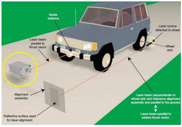
Operating statistics from long-haul truck companies have shown that collision warning and ACC systems can reduce accidents by as much as 70%. Until now installation and alignment of these systems during vehicle manufacture has been a costly, manual, time-consuming process even on the lowest-volume vehicle production lines.
